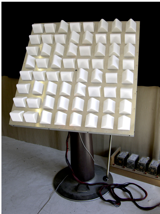
Fig 1. Board with 64 pluggable lamps
